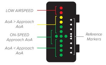
An Angle of Attack System is standard on all Skyhawks, delivering precise information for increased stall awareness, low-speed maneuvering capability and consistent maneuvers during takeoff, climb, cruise, approach and landing.
